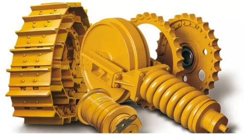
Bottom roller excavator is made of shell, bronze bushing, collar, seal, lock pin, plug, shaft. It is made by forging, machining, heat treatment, assembly, painting etc. The quality and working life for bottom roller excavator is depends on the quality of raw steels, the hardness of rail
